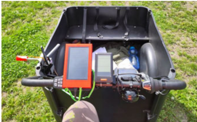
Figure 2 Driver point of view of the 5G-Hardware installed on the Cargo Bike. Author: Johan Levon.
